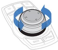
Turn the controller until the desired menu item is highlighted.
